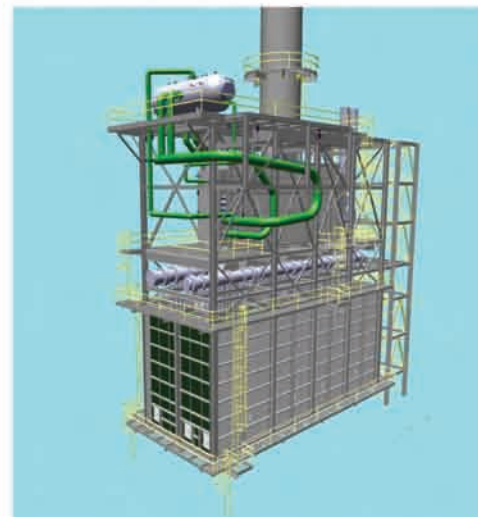
Steam superheater. The design tools utilized by SFPC allow clients to progressively visualize the furnace as it is being designed.
